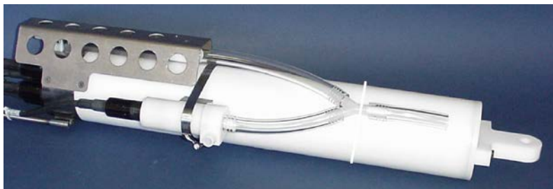
SBE 19plus V2 SeaCAT with SBE 5M plastic pump
